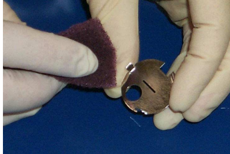
Figure 5-17 Discolored Ground Slit Plate
