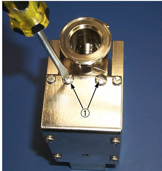
Figure 5-4 Slotted Screws that Attach the Magnet Assembly to Spectrometer
