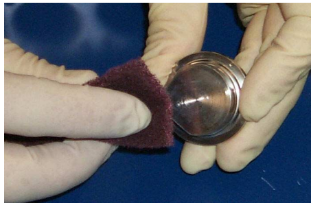
Figure 5-18 Discolored Ground Magnet Pole Piece
